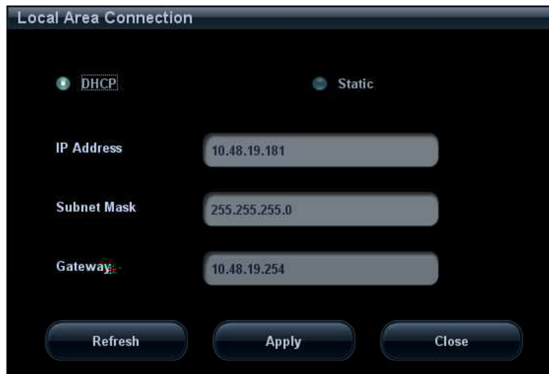
Figure 2 TCP/IP Local Area Connection Preset Screen
