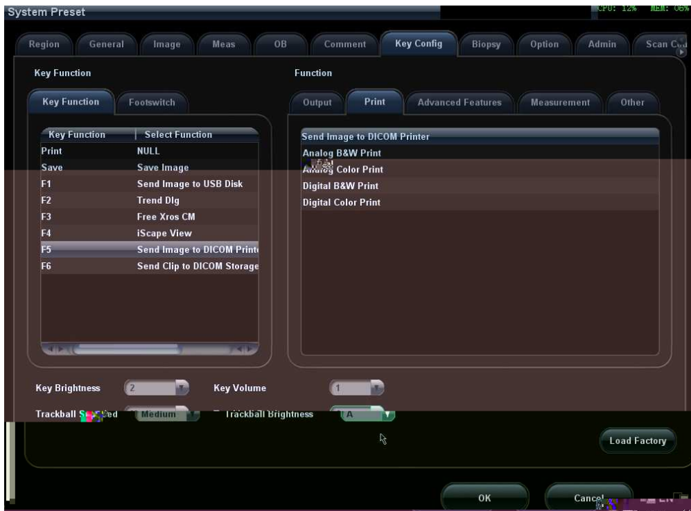
Figure 9 Send to DICOM print when pressing user-defined key
